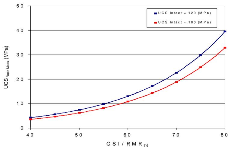
**Figure 4** Increase in  $UCS_{rock\ mass}$  with increasing GSI or RMR<sub>76</sub>
