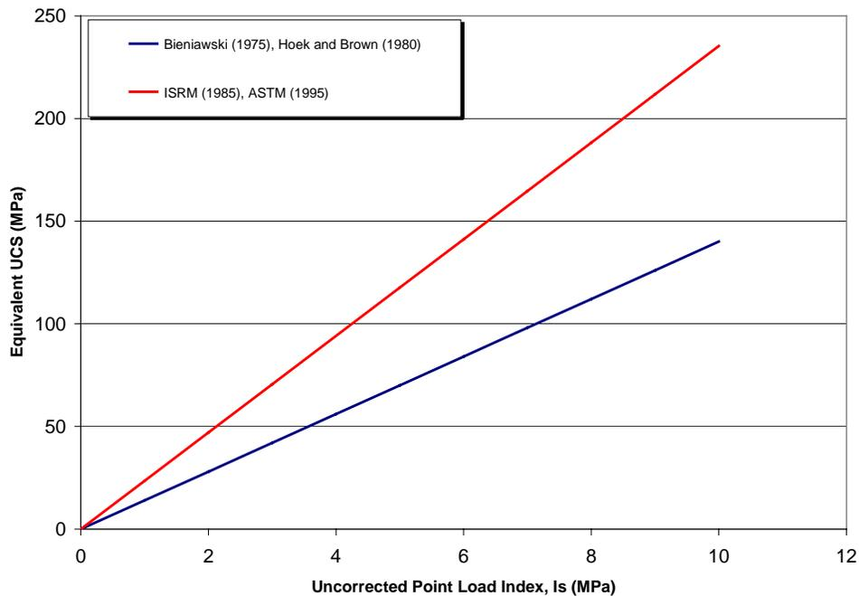
**Figure 3 Comparison between equivalent UCS obtained using the Bieniawski (1975) method and the current ISRM and ASTM methods assuming the default conversion factor of 24**
