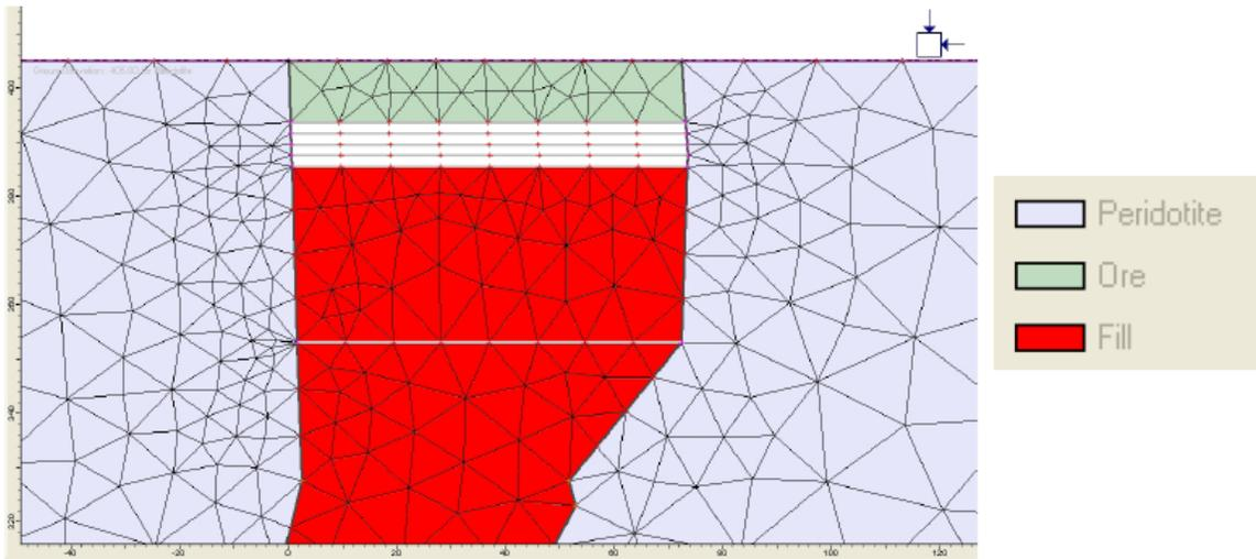
**Figure 6** *Phase<sup>2</sup> model geometry and finite element mesh (Golder, 2006c)*
